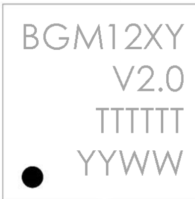
Figure 8.2. BGM121/BGM123 Package Marking
